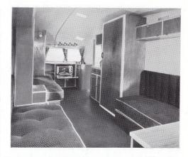
of the two single beds in the front apartment which can be separated from the rear of the caravan by folding doors. Valuable locker space is provided below the sink and cooker and storage space for a gas cylinder is available in the cupboard immediately adjacent to the doorway.
