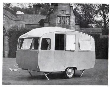
Designed for touring with the lower powered range of cars, the "Glendale", in the illustration above, shows to advantage the smooth exterior line and generous window area. Stable type door and full road lighting are desirable features common to all Thomson touring caravans. The caravan is mounted on  $4.75 \times 16$ " tyres.
