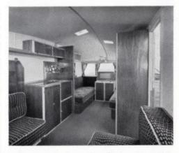
utensil storage and cutlery drawer are in the cupboard below the cooker. The table is stowed against the wall next the sink and behind the back rest of the dinette.
