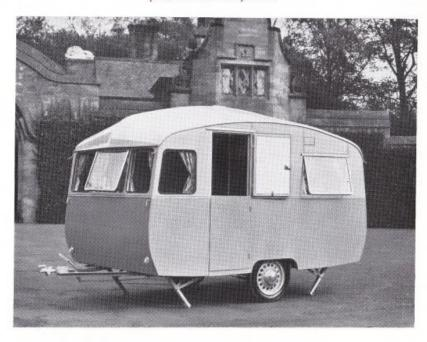
Designed for touring with the lower powered range of cars, the "Glendale", in the illustration above, shows to advantage the smooth exterior line and generous window area. Stable type door and full road lighting are desirable features common to all Thomson touring caravans. The caravan is mounted on  $4.75 \times 16$ " tyres.
