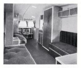
of the two single beds in the front apartment which can be separated from the rear of the caravan by folding doors. Valuable locker space is provided below the sink and cooker and storage space for a gas cylinder is available in the cupboard immediately adjacent to the doorway.
