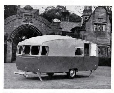
This illustration shows the graceful lines of the "Gleneagle" with its specially designed low overall height which also permits maximum interior headroom of 6' 4". The stable type door and telescopic jockey wheel are clearly seen and of special interest is the full width front window arrangement which is repeated at the rear with an opaque window in the toilet room. The "Gleneagle" chassis is rolled steel channel and carries  $6.00 \times 16''$  tyre equipment.
