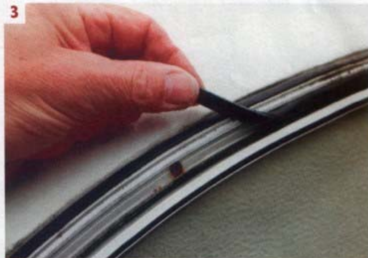
3 ■ Stage one was to peel away its plastic insert which is a cosmetic way to hide the screws
